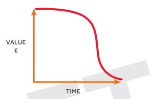
It can be seen that when a certain point is reached in time, the depreciation accelerates rapidly resulting in higher maintenance costs. The time for bitumen to age to reach this point is 10 years as defined in the TRL Report 24.
